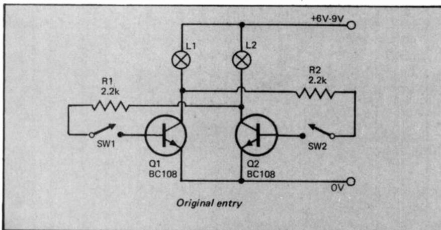
THIS CIRCUIT was thought up by Mr T. Tuck of Salisbury, South Australia. It's purpose is to indicate which of two switches is first depressed.
