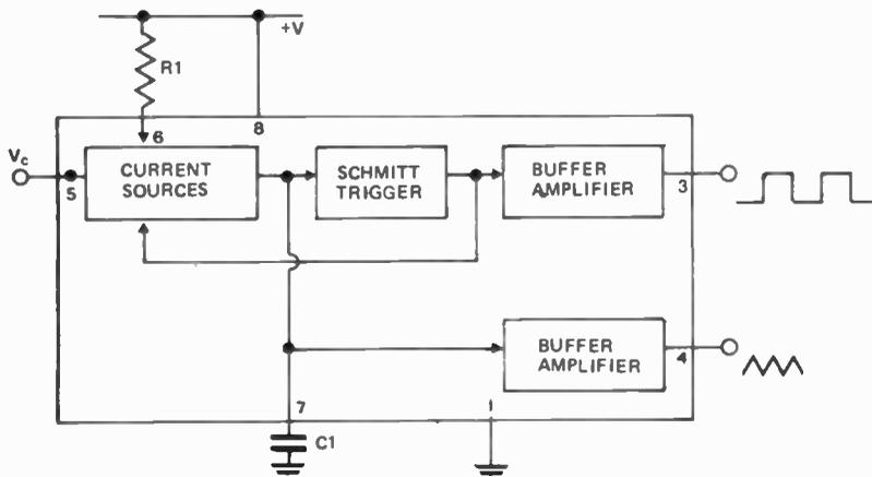
Fig. 2. Basic circuit of the NE566V in block form.
