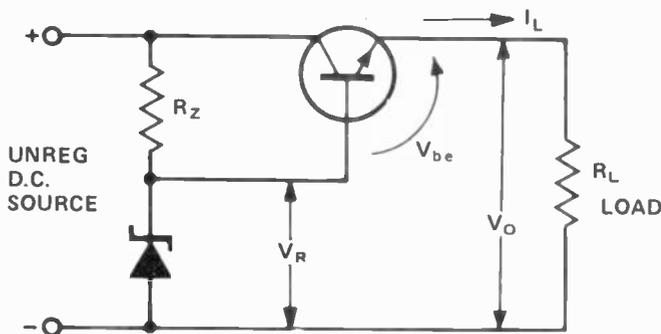
Fig. 11. The series regulator also relies on feedback to control voltage drop across a series-pass transistor.
