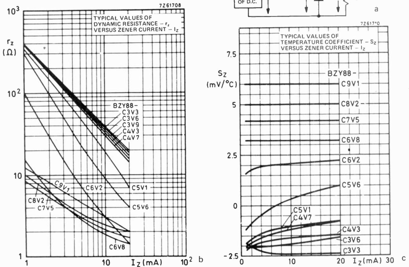
Fig. 6. (a) Typical Zener diode regulator. (b) dynamic resistance of BZY88 series Zeners. (c) temperature coefficients of BZY88 series diodes.
