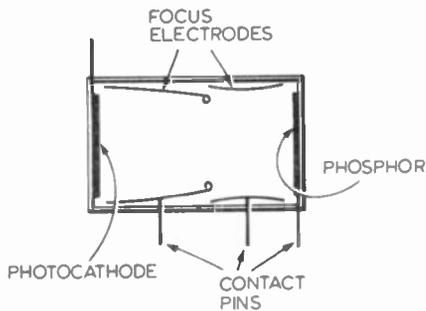
Fig. 4. Photocathode/phosphor cell.
