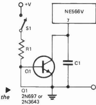
Fig. 8. A method of switching the oscillator on and off.
