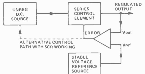
Fig. 9. Generalized diagram of active feedback type regulator.
