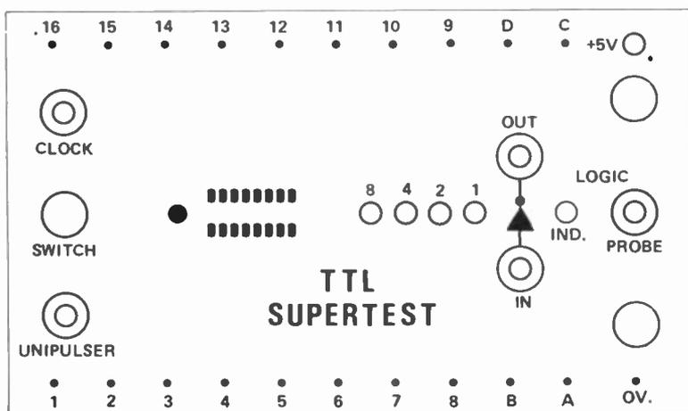
*Front panel layout of unit (with optional BCD readout). Use printed circuit board as guide for marking out hole centres etc.*
