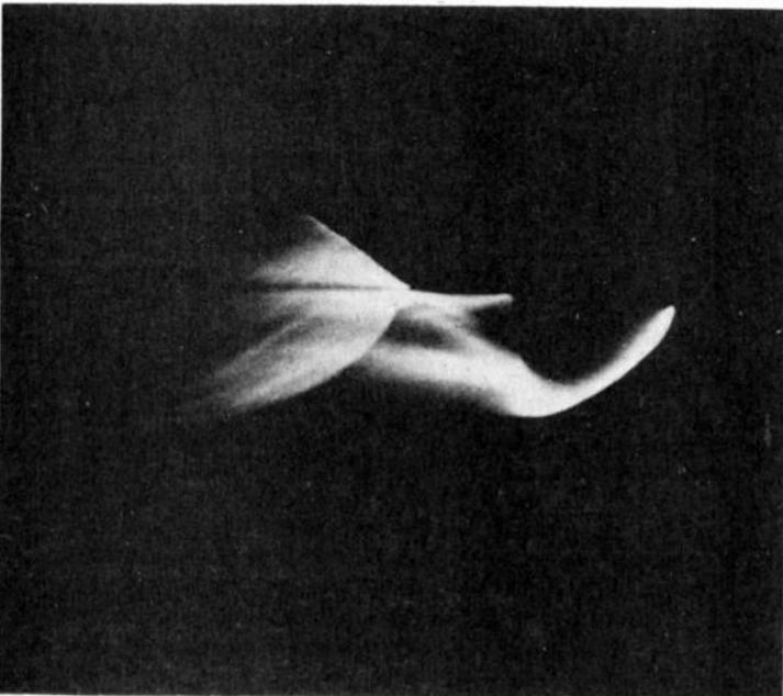
*Ultra-high-speed recording of a streak record of plasma formed in nitrogen by carbon dioxide TEA laser.*
