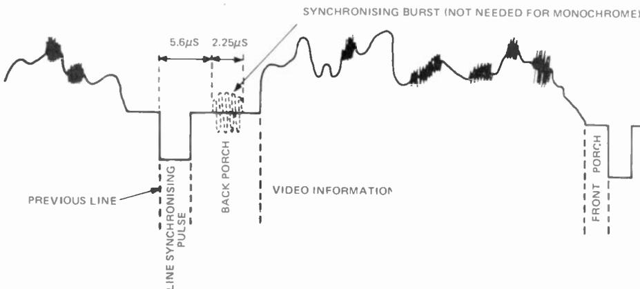
Fig. 24. Waveform of one line of a colour picture. A short 'burst' of unmodulated 4.43 MHz subcarrier is transmitted in the back porch period for reference oscillator synchronisation.
