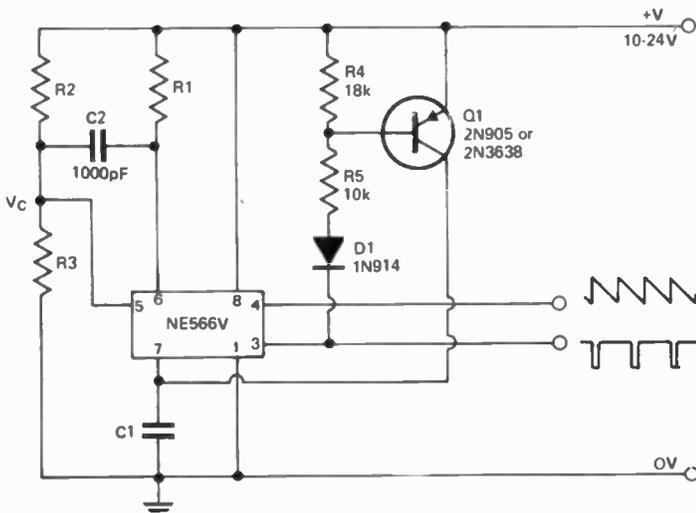
Fig. 6. Falling ramp generator.
