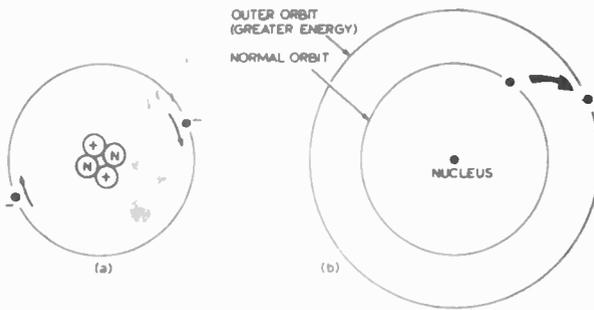
**Fig. 2. LEFT:** One way of visualising the atomic structure (see main text). The core consists of protons (+) and neutrons (N) with negative electrons/moving round it. **RIGHT:** If energy can be transferred to the electron, its orbit moves out. If it returns, the energy difference is released.
