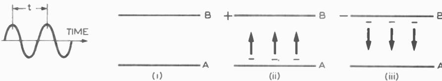
Fig. 1. Most electronic amplifiers depend on electrons (or holes) moving from some part (A) to another part (B). If (B) is positive, electrons move towards it, but if the signal at (B) is reversed before the electrons reach it electron movement will cease or be reversed.
