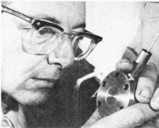
Cell from a sodium-sulphur battery is inspected by Dr. S. P. Mitoff. In background, a flame issues from the mouth of a furnace used in preparing the battery's ceramic electrolyte.
