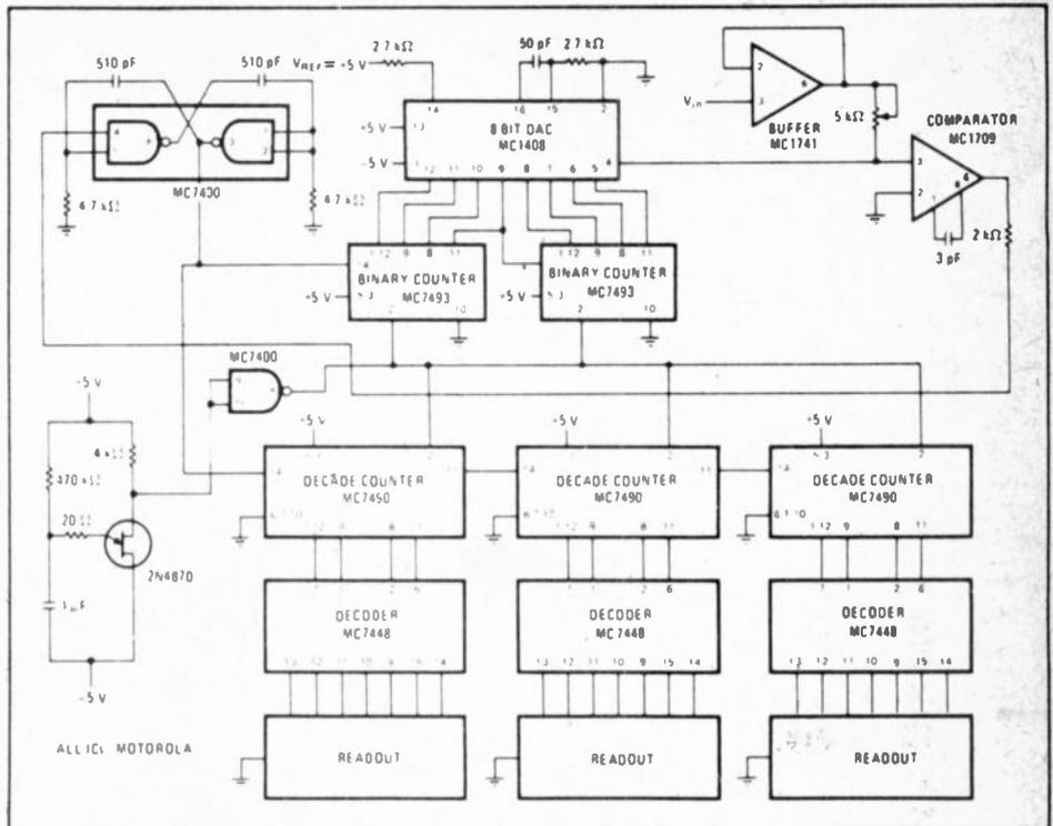
compared to the unknown input signal, and the clock pulses are terminated when the input signal level and the staircase function level are equal. The number of clock pulses occurring during the comparison process are therefore proportional to the voltage of the unknown input signal.
