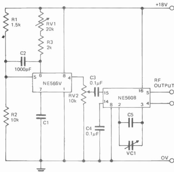
Fig. 9. A radio frequency f.m. generator.
