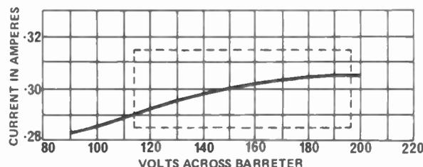
Fig. 2 (a). The barretter tube regulates by the increase in resistance with temperature (and hence current) of an iron-wire filament.
