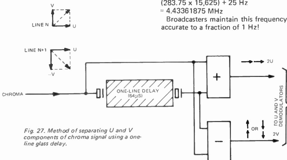
Fig. 27. Method of separating U and V components of chroma signal using a one-line glass delay.
