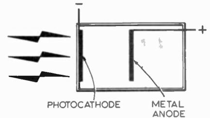
**Fig. 3. Construction of a simple photocell showing photocathode and anode.**
