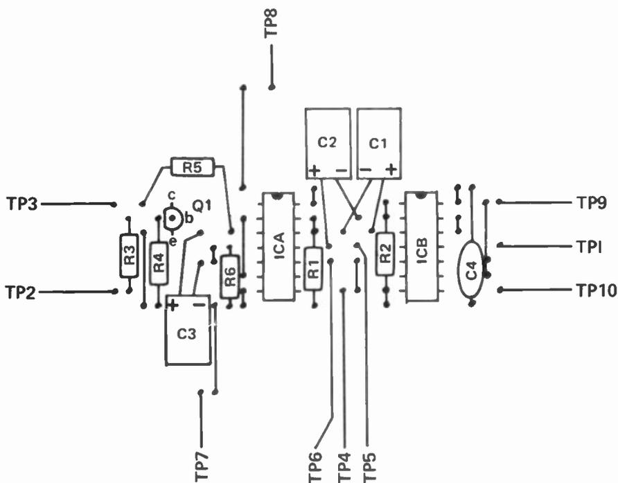
ORIGINALLY conceived as a tester for checking out disposals dual-in-line T.T.L. integrated circuits, this device has also proven effective in the roles of logic trainer, breadboarding unit and digital trouble-shooter.
