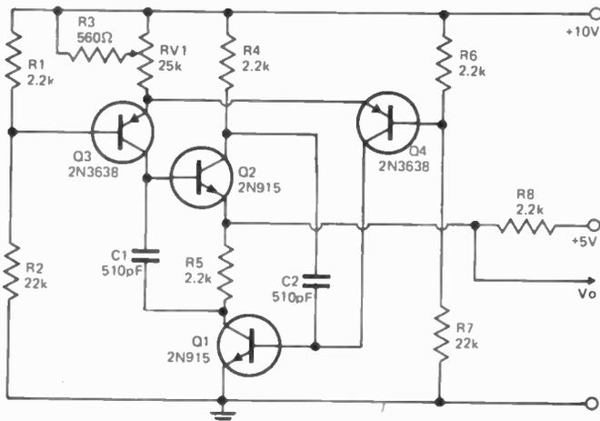
Fig. 2. Well-shaped variable frequency square-waves (5 kHz — 50 kHz) are supplied by this circuit, which is also capable of high frequency operation.
