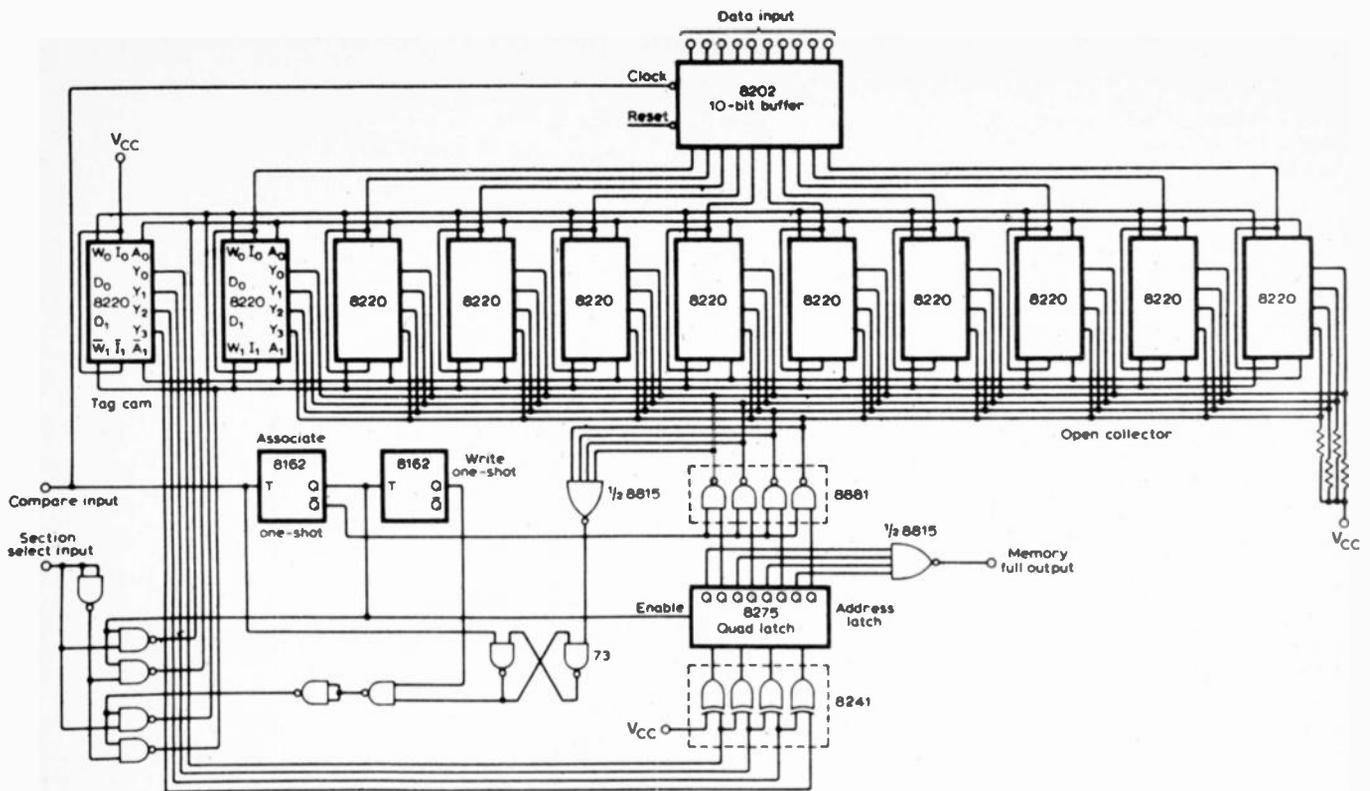
capacity of the memory is 80-bits (8 x 10), eleven CAMs are employed which together have a capacity of 88-bits (11 x 2 x 4). The eleventh CAM has been called the tag CAM because it keeps track of the locations within the memory which are occupied, and allocates a new address for acceptable information.
