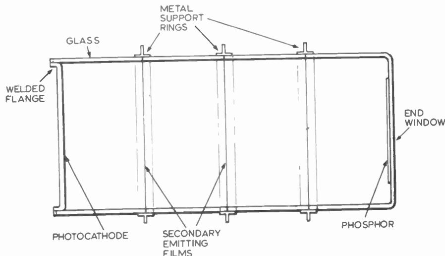
Fig. 6. Secondary emission intensifier.
