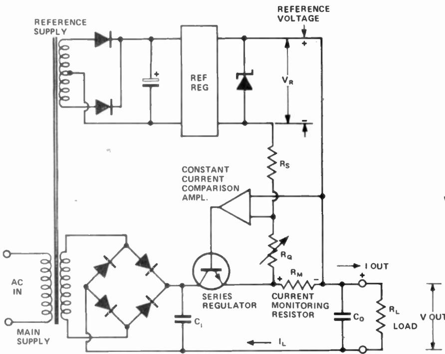
Fig. 13. Constant-current control is easily obtained as an extension of the constant-voltage supply. A series sensing resistor produces a voltage which, in conjunction with an error amplifier, controls the series pass transistor to maintain constant current.
