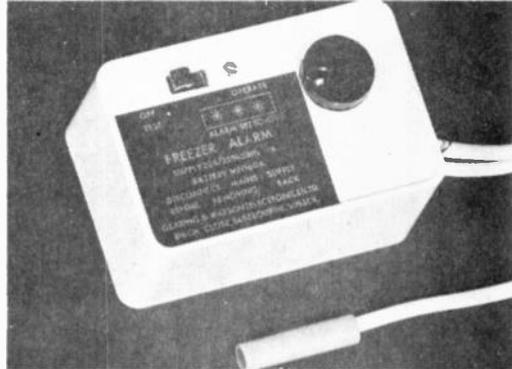
Gearing & Watson (Electronics) Ltd of the United Kingdom, manufacturers of process control equipment have released a device which may be incorporated with freezers at point of manufacture or may be installed in freezers already in use, by the owner without the use of tools.
