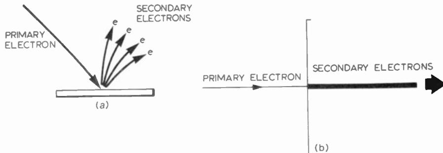
Fig. 5. Secondary emission of electrons by reflection (a); secondary emission by transmission (b).
