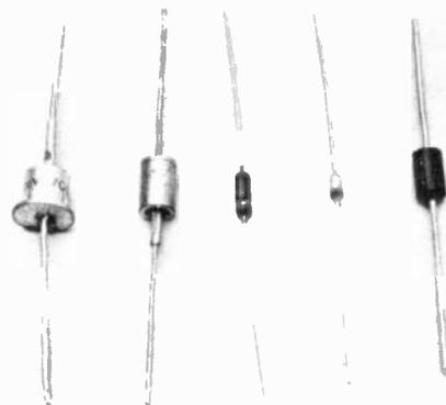
Fig. 5. Zener diodes are manufactured in a wide variety of packages. The larger capacity (not shown here) units are usually mounted on heat sinks if run at their maximum rating.
