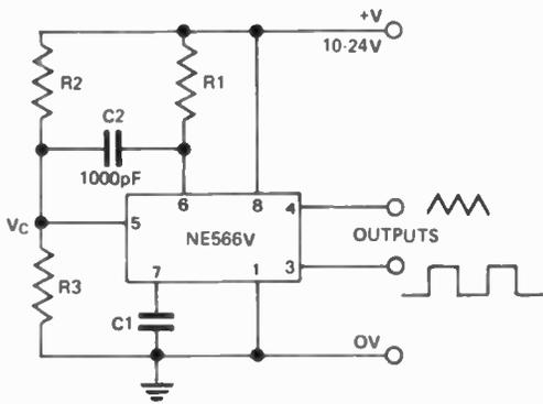
Fig. 5. Basic circuit for using the NE566V.
