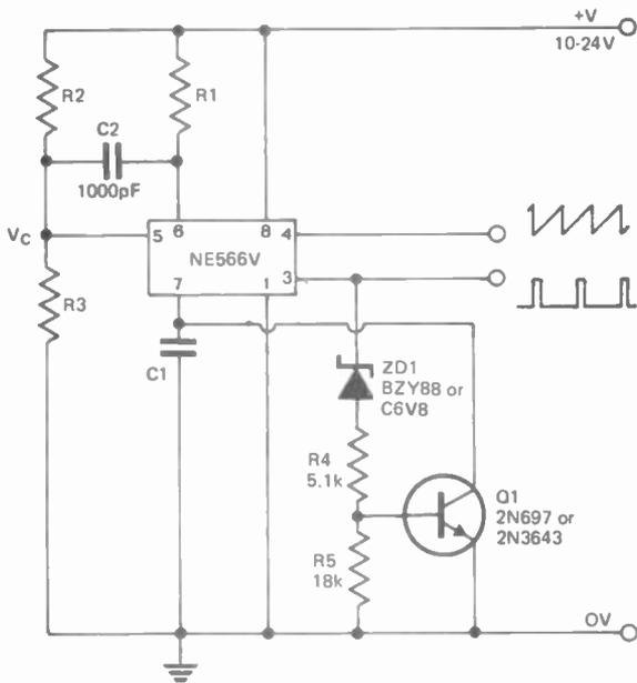
Fig. 7. Rising ramp waveform generator.
