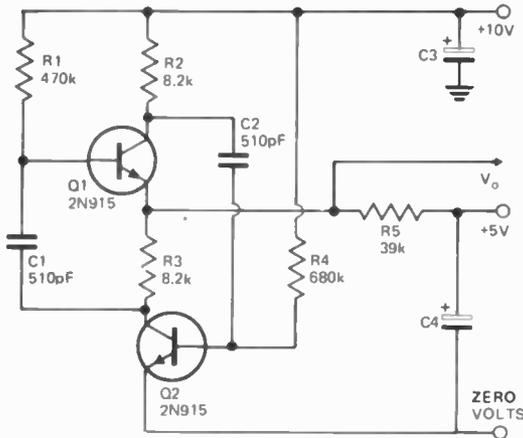
Fig. 1. This circuit supplies well-shaped square-waves.
