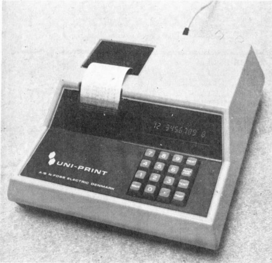
Foss Electric have introduced a printer designed for use in data handling where print-out, manual entry and additional information, automatic numbering and visual control of data are required. The printer can act as an interface for transference of data to storage.
