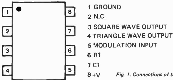
Fig. 1. Connections of the NE566V.
