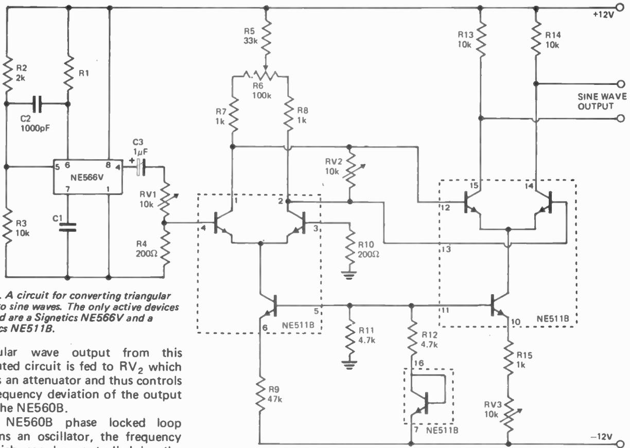
Fig. 10. A circuit for converting triangular waves to sine waves. The only active devices required are a Signetics NE566V and a Signetics NE511B.
