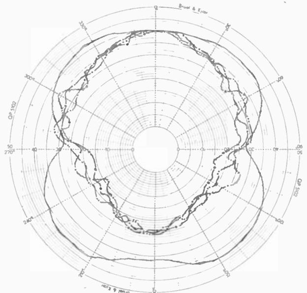
Horizontal pattern at two metres (input, one-third octave filtered pink noise). [1 kHz - . . . .], [4 kHz - . - . -], [8 kHz - - - - -], [16 kHz - o - o - o].
