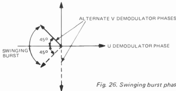
Fig. 26. Swinging burst phases.
