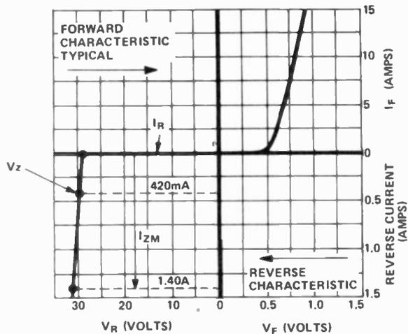
Fig. 4. In a zener diode the reverse-breakdown region is used to provide a constant voltage as current demand varies.
