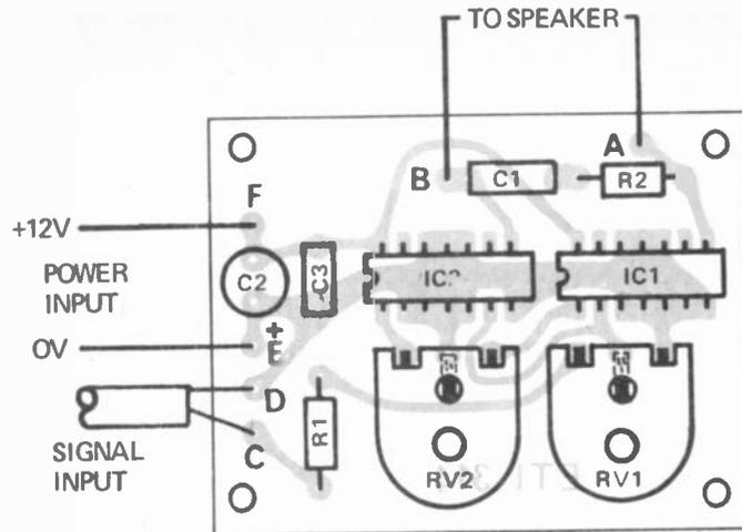
Fig. 3. Component overlay.
