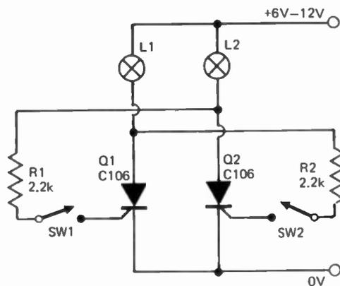
The circuit is self-latching if the transistors are replaced by SCR's.
